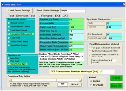
This screen opens when you start "Servo Test" from main menu. (For Servo Controlled m/c)
